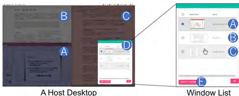
Figure 8: Sharing Application Windows Using USB Memory.
